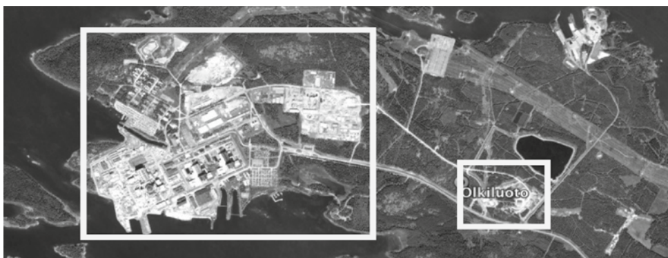
Figure 7.2. Surface facilities at Finland's planned Onkalo Repository, 2010. Coordinates N 61° 14' 10", E 21° 28' 50". The repository facilities occupy an area of about 0.25 km 2 (the small white rectangle on the right), one sixteenth that of the reactor site which hosts two operating reactors and one under construction (the white rectangle on the left). Source: Satellite image by Digital Globe/Google Earth, 31 May 2010.
