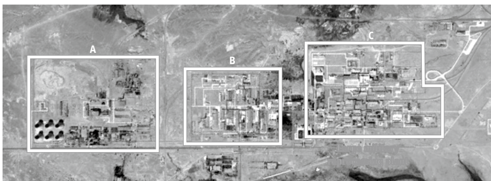
Figure 2.3. Jiuquan nuclear complex. Satellite image from 18 July 2011. Coordinates N 40° 13' 48", E 97° 21' 50". Box A envelopes the shutdown plutonium production reactors; Box B envelopes the small military reprocessing plant; and Box C envelopes the large military reprocessing plant and civilian pilot scale reprocessing plant. Source: DigitalGlobe and Google Earth.
