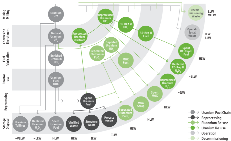
Figure 3.2: Generation of different radioactive-waste streams by nuclear power in France. Source: WISE-Paris.
