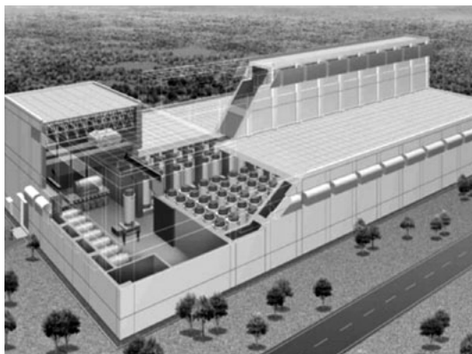
Figure 12.3: Artist's conception of a 3,000-ton-capacity interim dry-cask storage facility under construction in Mutsu in Aomori Prefecture, Japan near Japan's Rokkasho reprocessing plant. The outer walls provide additional radiation shielding and protection against projectiles. The purpose of the high structure running down the middle of the building is to increase the convective flow of warm air out of the building through the "chimney effect." 505 Source: Hitachi-GE Nuclear Energy Ltd.
