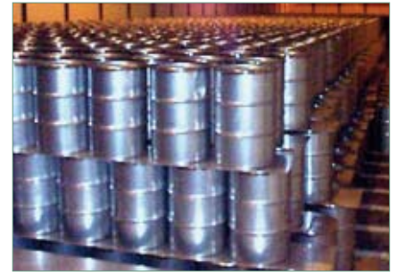
The storage of uranium oxide material is in stainless steel drums each weighing 600kg.
