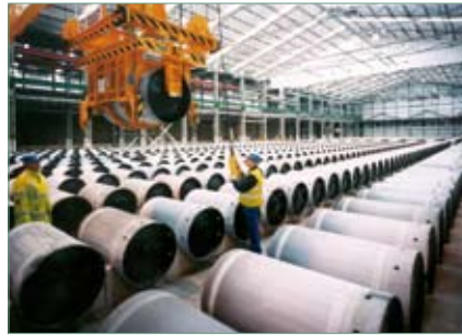
The current storage arrangement for uranium hexafluoride cylinders is in rows stacked up to five high.
