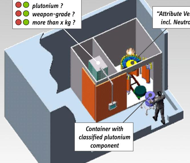
"Attribute Verification System" (AVNG) incl. Neutron and Gamma Detector
