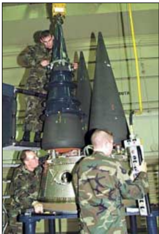
Munitions specialists from the 90th Maintenance Squadron at F.E. Warren Air Force Base, WY, work on the 3 RVs of a Minuteman III ICBM (USAF Photo, August 2001)
