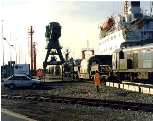
Figure 3. Spent Fuel Transport. Whilst UK spent fuel is transported in 50 ton cuboid flasks secured inside rectangular steel transport cabins, overseas fuel arrives in the UK in cylindrical flasks - typically in Excellox, Castor or TN flasks weighing up to 100 tons, and is transported uncovered on the rail journey to Sellafield. The rail link and casks were identified as a target by the IRA in the 1980's. Source: CORE archive
