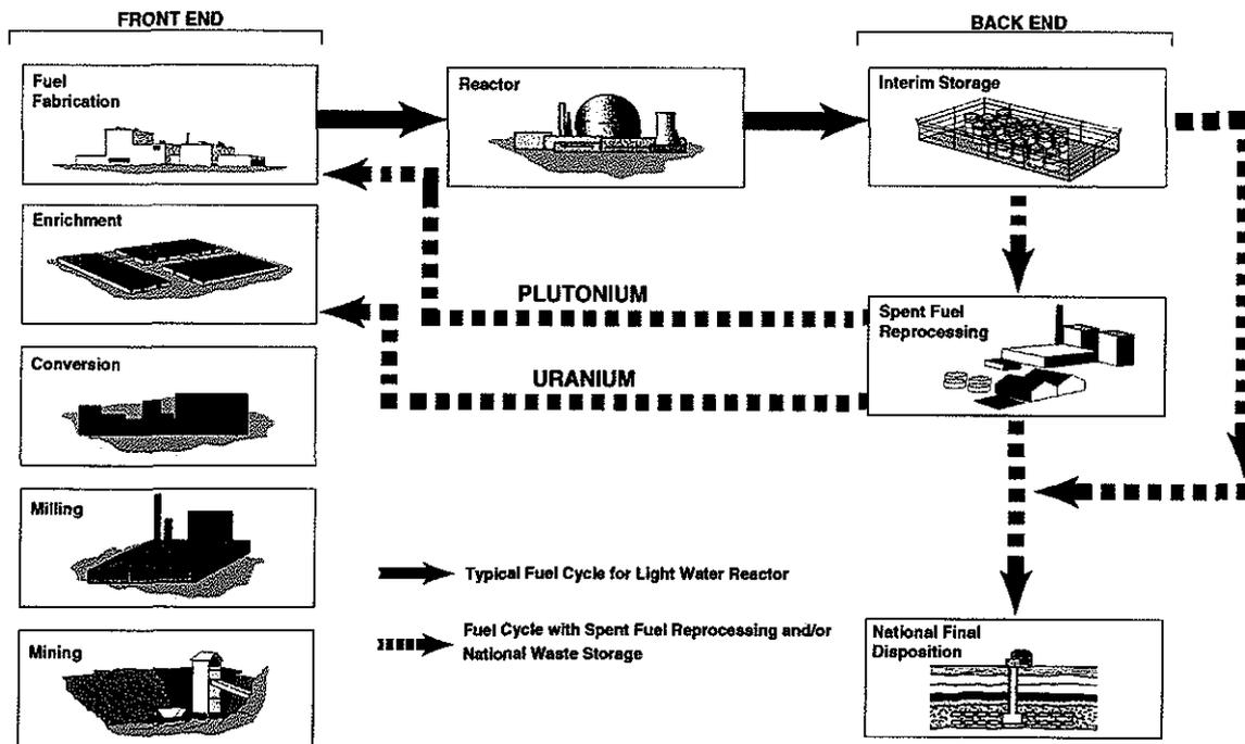
Fig. 1. The nuclear fuel cycle.
