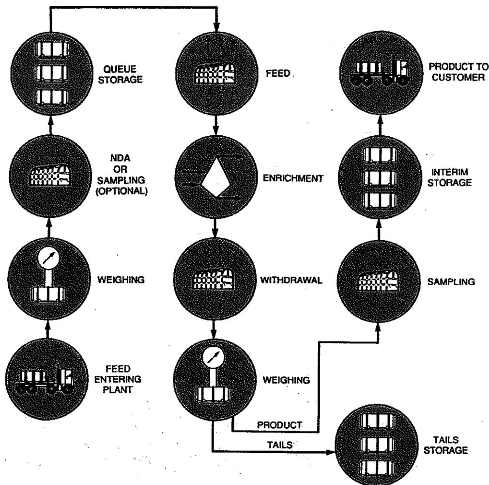
Fig. 28. UF<sub>6</sub> operations in an enrichment plant.
