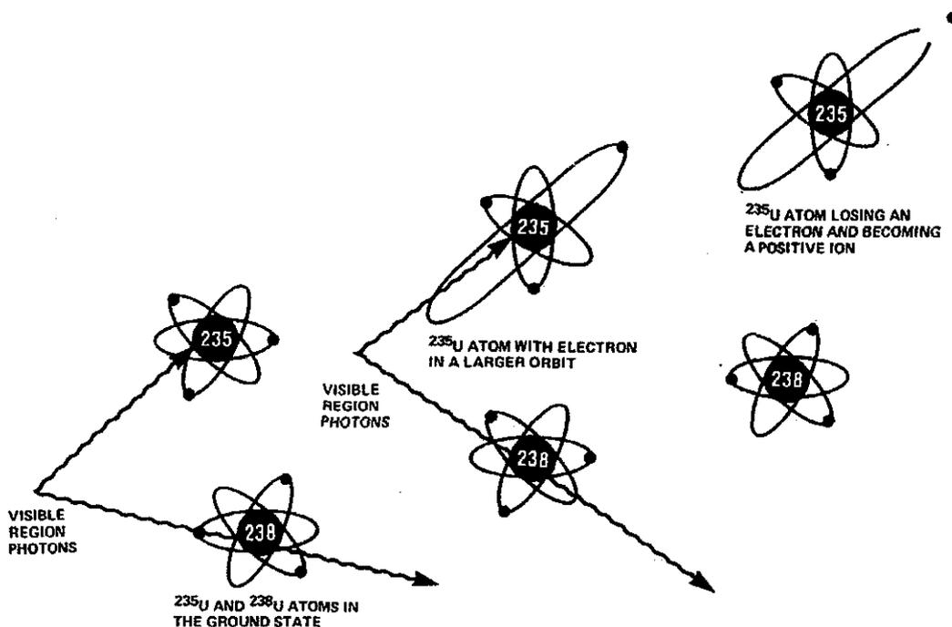
Fig. 12. Atomic vapor laser isotope separation process.
