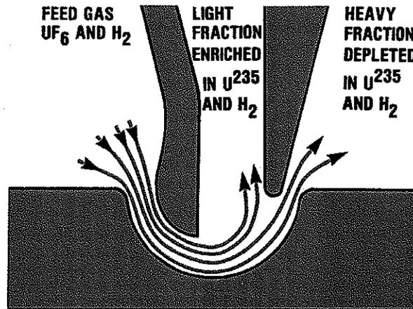
Fig. 8. Separation nozzle process.
