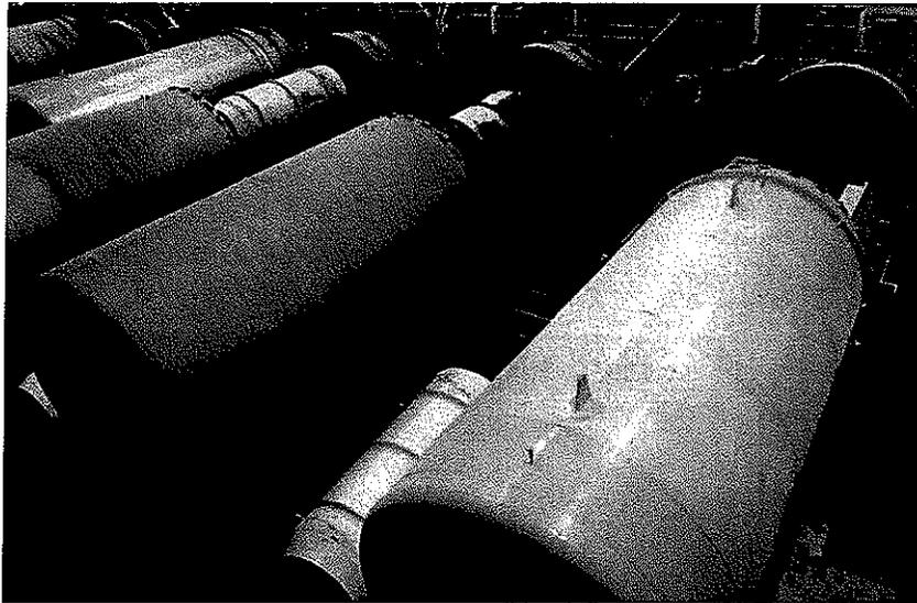
**Fig. 35. Steam autoclaves for  $\text{UF}_6$  feeding.**
