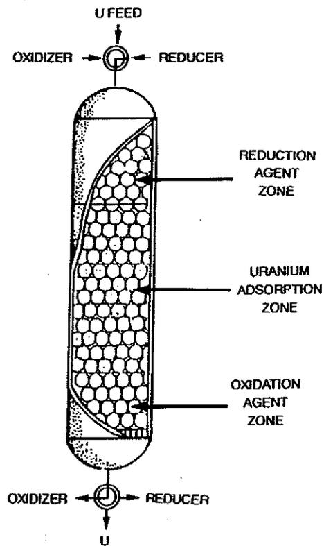
Fig. 11. Ion exchange process.
