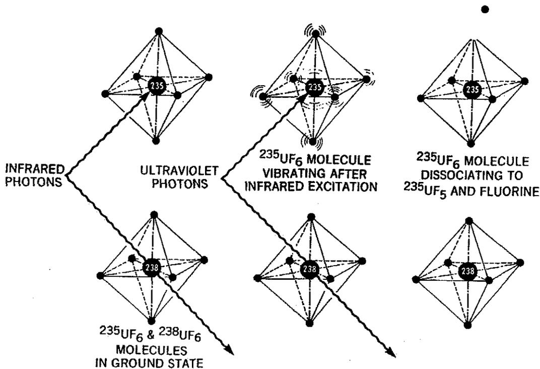
Fig. 13. Molecular laser isotope separation process.
