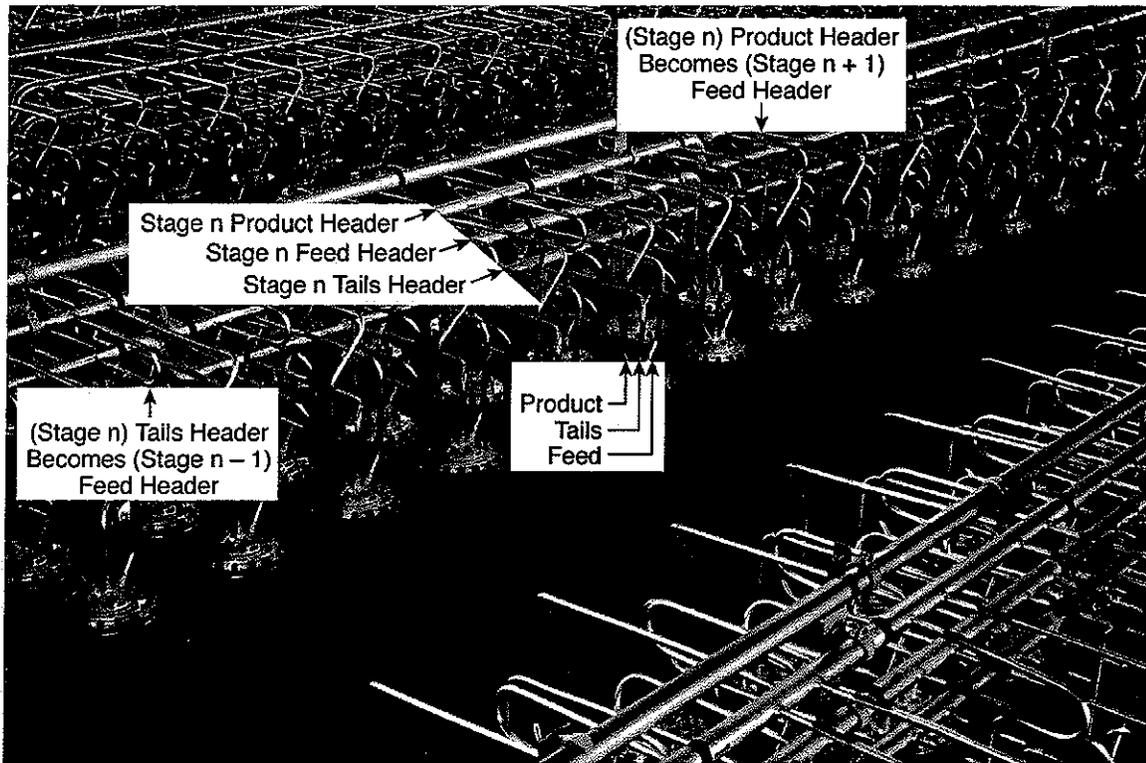
Fig. 27. Stage header piping in centrifuge cascade.
