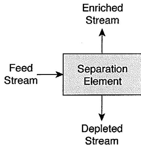
Fig 2. Basic separation element.
