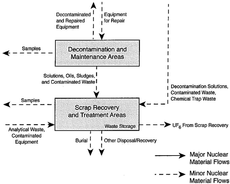
Fig. 24. Nuclear material flows at a typical gas centrifuge enrichment plant.
