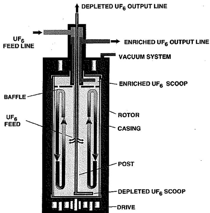
Fig. 6. Schematic diagram of a gas centrifuge.
