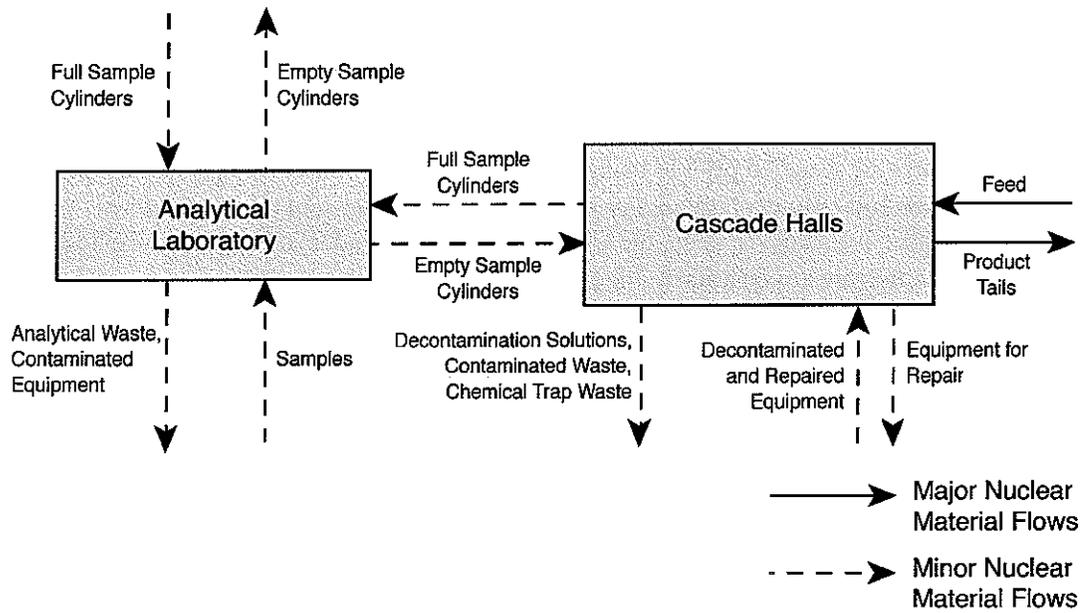
Fig. 23. Nuclear material flows at a typical gas centrifuge enrichment plant.
