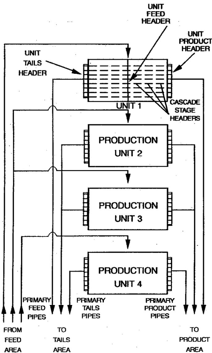
THE CENTRIFUGES IN UNIT 1 PROVIDE A QUANTITY OF MATERIAL AT A SPECIFIC PRODUCT ASSAY.
