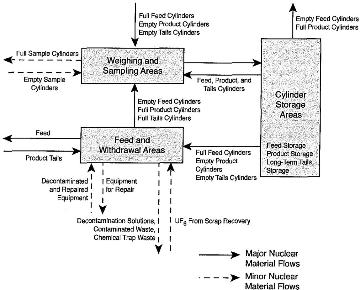
**Fig. 22. Nuclear material flows at a typical gas centrifuge enrichment plant.**
