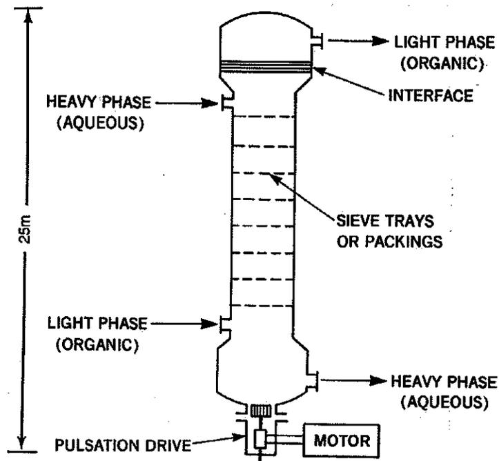
Fig. 10. Chemical exchange process.
