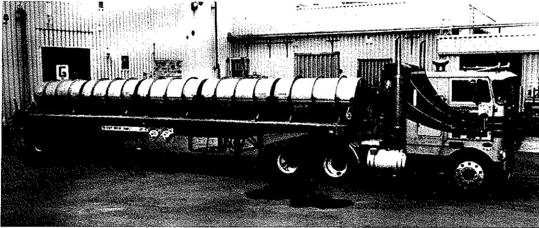
Fig. 29. Truck shipment of five 2 1/2-ton UF<sub>6</sub> cylinders in protective shipping packages.
