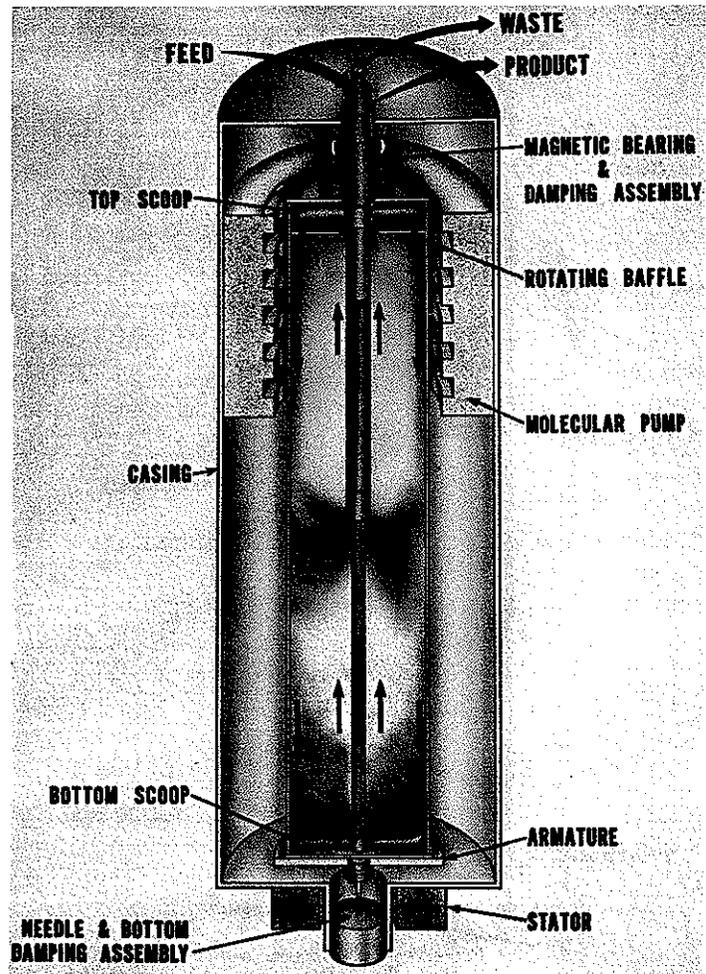
Fig. 17. Modern gas centrifuge.
