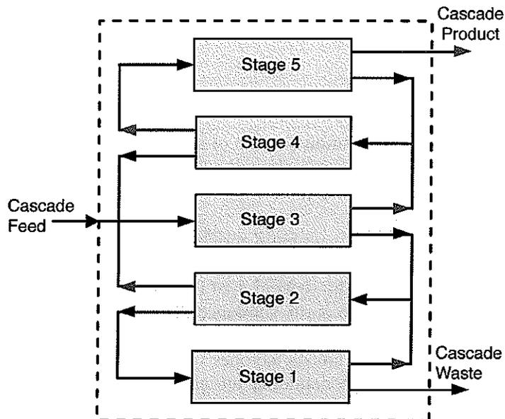
Fig. 3. Stages are connected in series to multiply the separation effect.
