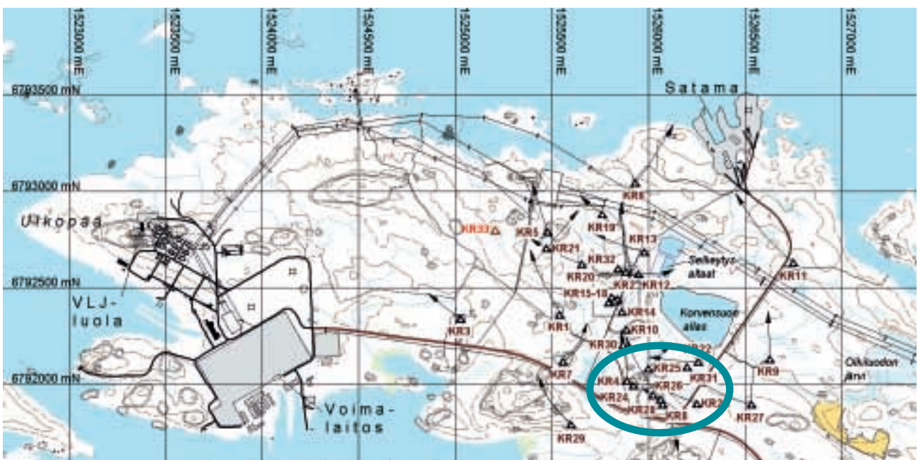
The map shows the location of ONKALO at Olkiluoto. Numerous deep boreholes were drilled in the investigation area to obtain further information for planning ONKALO.
